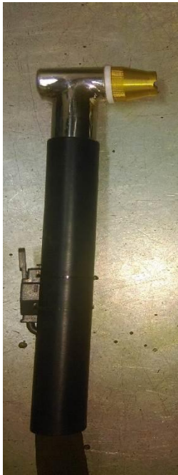
Air cooled Hand torch with Trigger lock Switch
